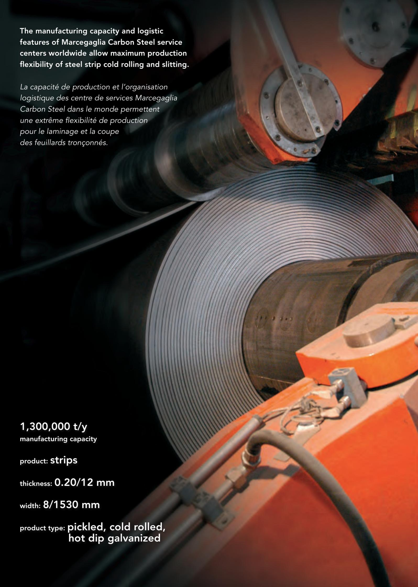
The manufacturing capacity and logistic features of Marcegaglia Carbon Steel service centers worldwide allow maximum production flexibility of steel strip cold rolling and slitting.
